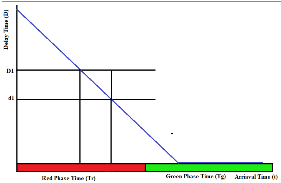
Figure 3.12: Changing Delay Time at Intersection
